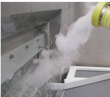
Abströmung in Steriltunnel Flow into Steriltunnel
